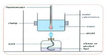
i) — Calculate the heat change of the reaction during the experiment. ( $Q = mc\Delta T$ )?
