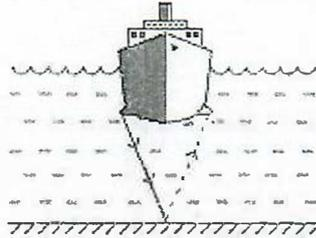
A wave is sent out from the boat to the sea bed and is received back 3 seconds later.
